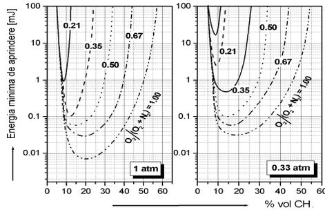
Figure 1. Variation of minimum ignition energy with pressure and gas composition for an oxygen-methane mixture.
