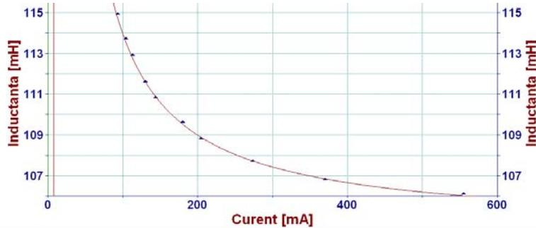
Figure 4. Inductance-current calibration curve
