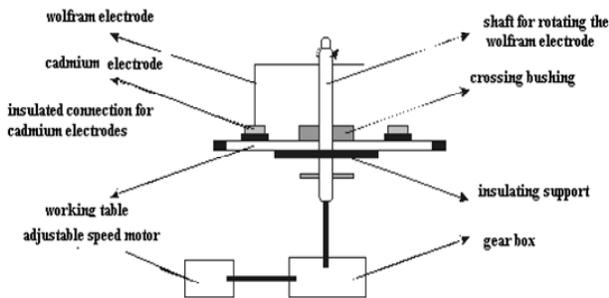
Figure 2. Explosion cell for the determination of the minimum ignition current
